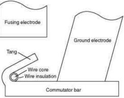
Figure 2: Commutator Fusing Process
